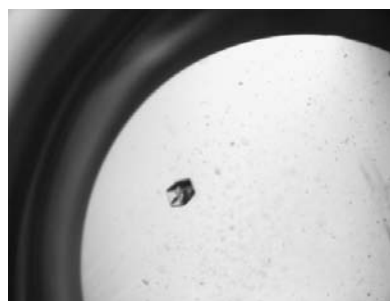
Figure 1 An orthorhombic crystal of a putative DNA methyltransferase from H. pylori (gene HP1352). The crystal dimensions are 0.3 \times 0.2 \times 0.2 mm. It diffracts X-rays to at least 2.5 Å resolution.
